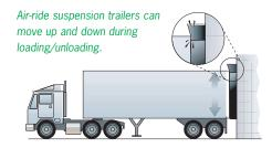
When a stationary head pad and wear pleat system is utilized, after time, movement of the trailer causes damage and can lead to detachment resulting in an unprotected wall surface and loss of seal.
