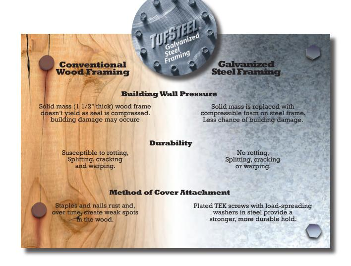
Tufsteel<sup>®</sup> Galvanized Steel Framing delivers low cost of ownership through durability and value. Kelley backs all Tufsteel framing with a 5-year warranty!
