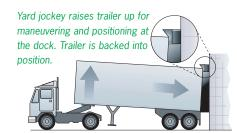
Wearmaster's two-piece floating head pad and wear pleat system accommodates movement as trailer is lowered.
