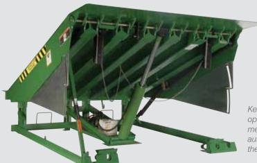
Kelley's HP dock leveler provides automatic hydraulic operation with a single push-button activation and a mechanically activated lip. The HP's unique Gravity-Lip  $^{\rm TM}$  automatically extends the lip in a smooth, quiet fashion as the dock leveler descends into the trailer.
