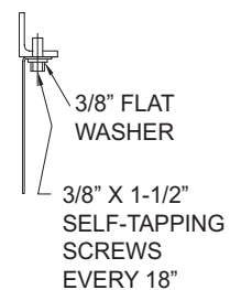
MOUNTING BRACKET TO STRUCTURAL STEEL
