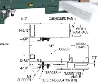
FILTER, REGULATOR, LUBRICATOR (FRL)—Filter, dual regulator, lubricator with safety shut-off valve, % in. NPT inlet port.
